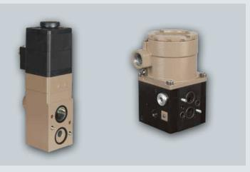
Solenoid valves serve as switching elements for the opening and closing of the valve assembly or act as safety control circuits for connected valve accessories to form the interface between the electric control level and the pneumatic actuator.
