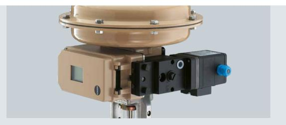
**Explosion protection** – The switching function in the solenoid valves is performed by an electropneumatic binary converter, which has proven reliable in service a million times over. Thanks to its low power consumption, the type of protection intrinsic safety (Ex i) is possible. Further available types of protection include flameproof enclosure (Ex d) and non-sparking equipment (Ex n).
