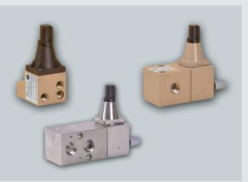
Lock-up valves are used to shut off the signal pressure line of pneumatic actuators. They shut off the line either when the air supply falls below an adjusted limit or in case of complete air supply failure. This causes the actuator to fail in place.
