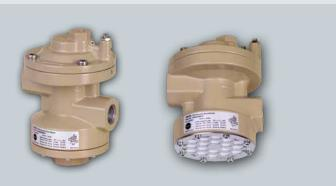
Volume boosters are used together with positioners to increase the positioning speeds of pneumatic actuators. They influence the process to vent or fill the actuator with air, which causes the control valve to open or close more quickly.
