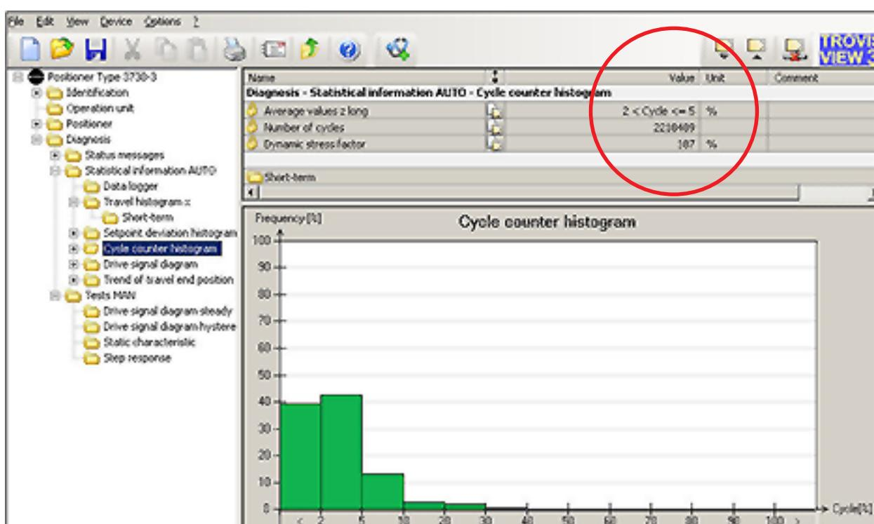
Figure 7.3.5.11.-3: Cycle counter histogram with TROVIS VIEW
