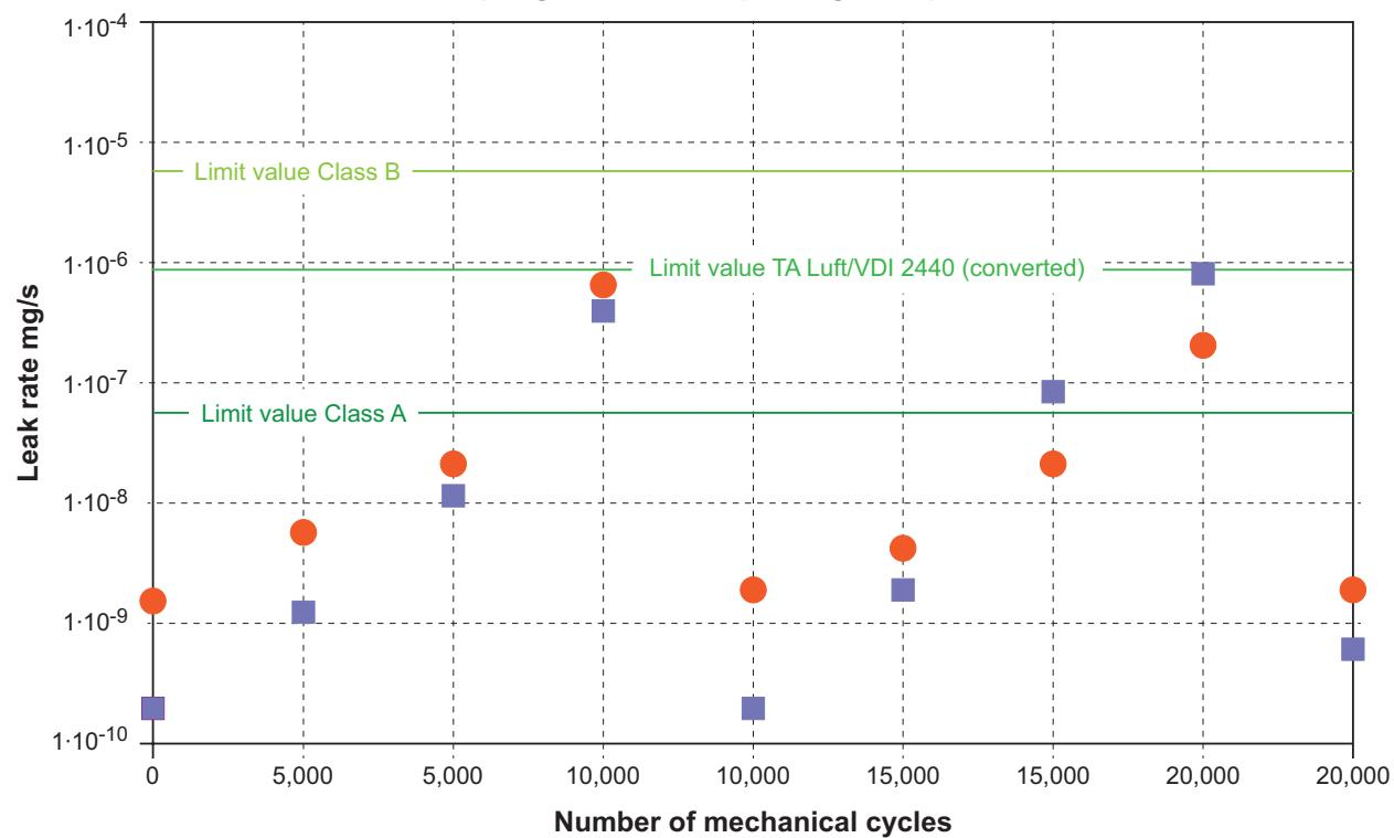
Figure 7.3.5.11.-5: Class CC1, spring loaded PTFE-packing, Test pressure 160 bar He
