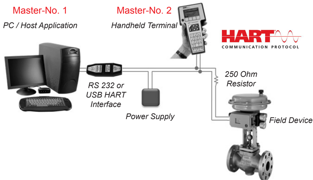
Figure 15.3.1.-3: HART® communication with two masters
