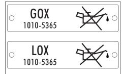
Fig. 1: Labels for gaseous oxygen (GOX) and liquid oxygen (LOX)
