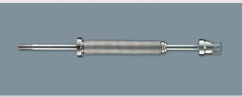
Metal bellows are used in globe valves to seal the plug stem to the atmosphere. The thin-walled corrugated cylinders are used as dynamic seals, particularly in applications where strict emission requirements apply. Metal bellows by SAMSON are made of corrosion-resistant materials. They are capable of withstanding high pressures and temperatures, which makes them ideally suited for use in high-performance service.
