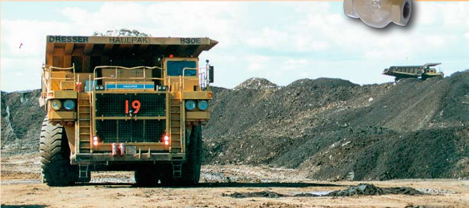
Gigantic off-highway trucks can carry loads of up to 400 tons, transporting the oil sands from the extraction sites to the processing facilities. · The Type 3525 Dump Valve is a low-cost solution for severe operating conditions in oil and gas plants.
