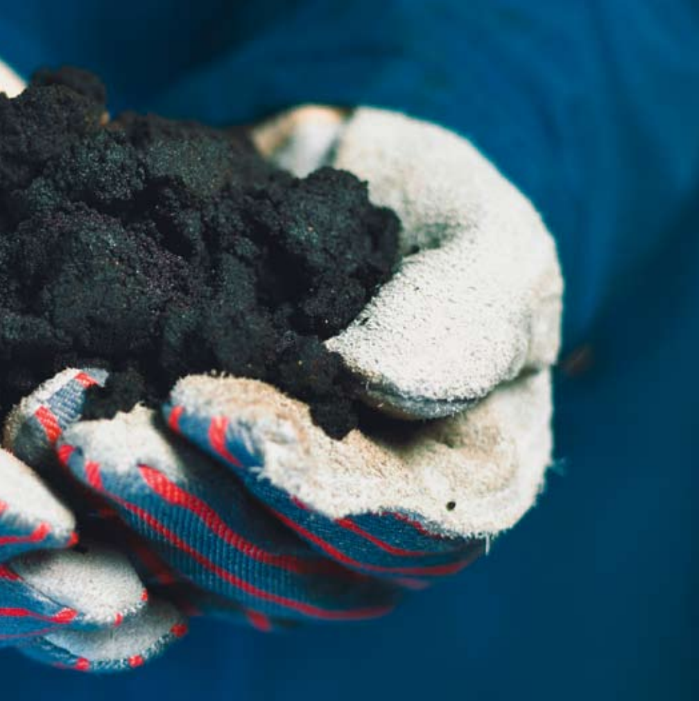
Alberta's oil sands contain about 10 % of bitumen. Sand, clay and water make up the rest of the sticky black mass.
