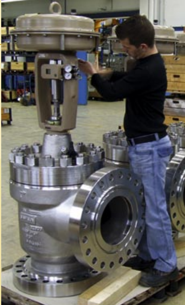
Final assembly of a stainless steel angle valve in DN 300 for the Puguang natural gas purification project in China.
