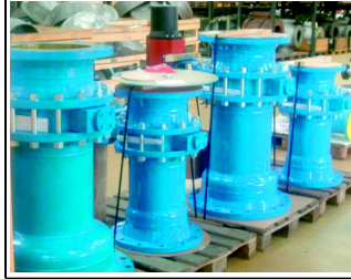
Fig 32b: Cooling water supply valve
