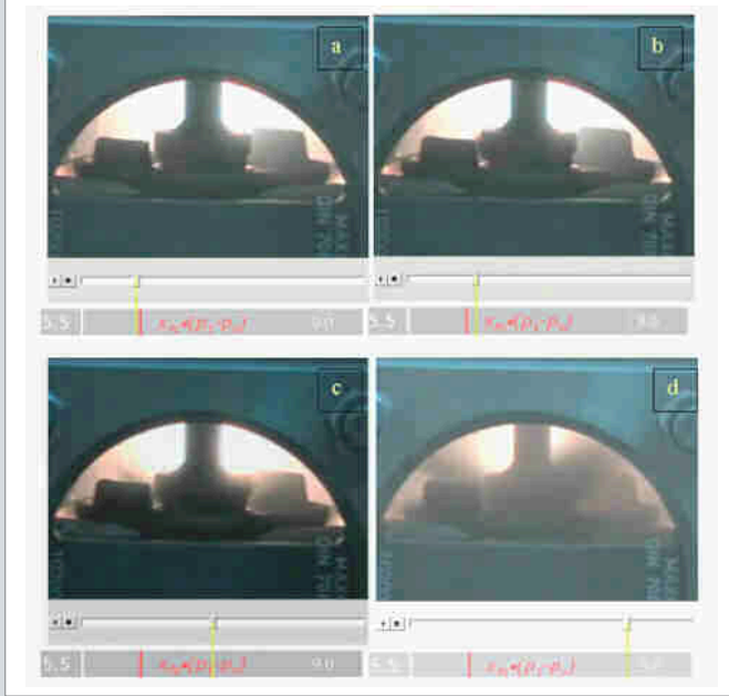
Fig. 2: Cavitation process in a control valve as a function of a pressure drop between 5.5 and 9 bar ( p_1 = 10 bar, p_v = 0.02 bar, water)
