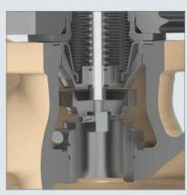
Special plug stem guiding for use in vertical pipelines
