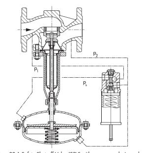
Type 33-1 Safety Shut-off Valve (SSV) with pressure reducing valve
