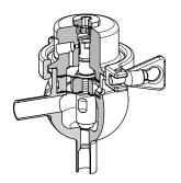
Type 2371-00 Pressure Regulator with pneumatic set point adjustment
