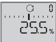
Initialization successful, positioner in automatic operating mode
