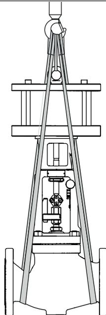
Fig. 4-4: Lifting points on the control valve (example)
