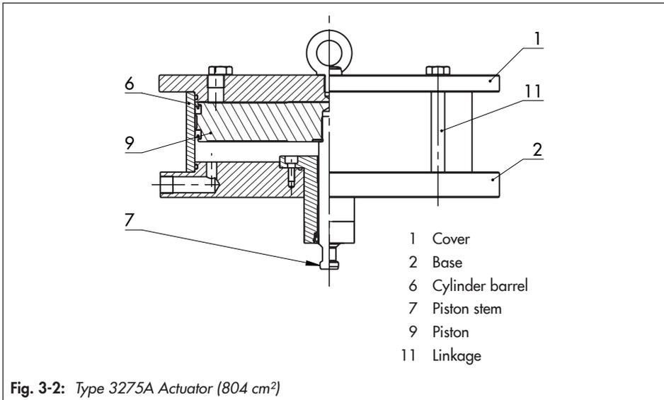
The actuator with 804 cm<sup>2</sup> area does not need a yoke (see Fig. 3-2). The valve accessories are mounted over the NAMUR interface.
