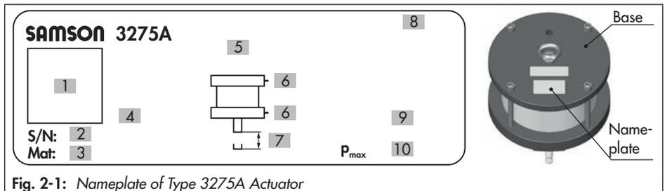
Fig. 2-1: Nameplate of Type 3275A Actuator
