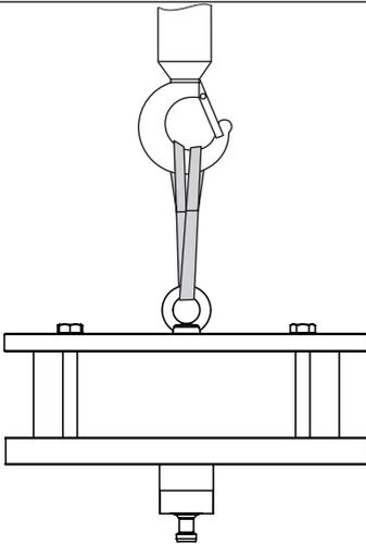
Fig. 4-3: Lifting point on the actuator
