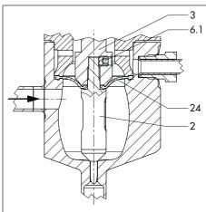
Fig. 9-4: Threaded pin on the plug stem/plug
