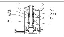
Fig. 9-1: Packing (with Type 3271/3277 Actuator)
