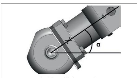
Fig. 2: Mounting position for self-draining of food processing valves
