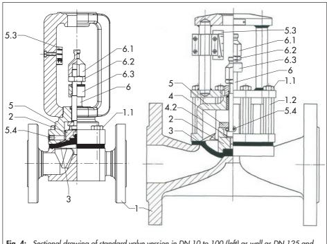
**Fig. 4:** Sectional drawing of standard valve version in DN 10 to 100 (left) as well as DN 125 and 150 (right)
