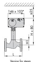
Type 3213/5724-3: DN 15 to 50 Type 3213/5724-8: DN 15 to 50 Type 3213/5725-3: DN 15 to 50 Type 3213/5725-8: DN 15 to 50
