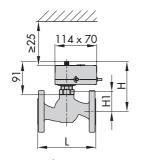
Type 3213/5857: DN 15 to 25 Type 3213/5757-3: DN 15 to 25 Type 3213/5757-7: DN 15 to 25
