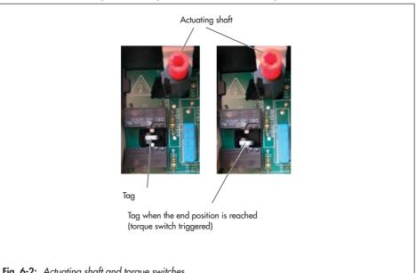
Fig. 6-2: Actuating shaft and torque switches
