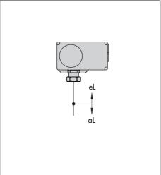
Fig. 8-1: Movement of the actuator stem
