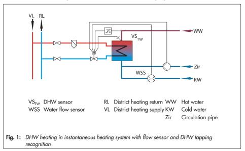
The DHW temperature is controlled to the set point temperature in DHW heating in instantaneous heating systems:
