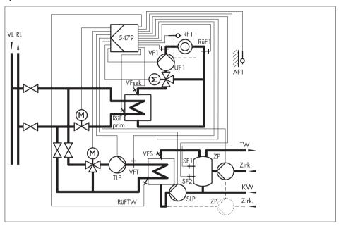
Set  $Co4 \rightarrow Fb11 = ON$  if the instrumentation represented by the broken line is required.
