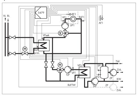
Set Co4 -> Fb11 = ON if the instrumentation represented by the broken line is required.
