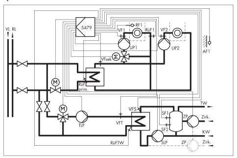
Set Co4 -> Fb11 = ON if the instrumentation represented by the broken line is required.
