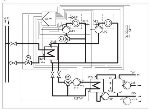
Set Co4 -> Fb11 = ON if the instrumentation represented by the broken line is required.
