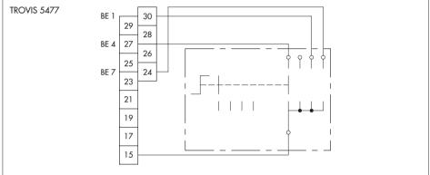
Fig. 23 · Example for the selection of the operating mode with an external switch
