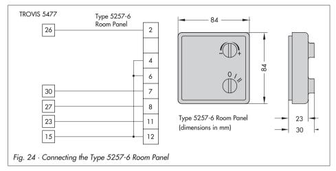
It is possible to use the room panel to correct a temperature set point or to select an operating mode when it is wired as shown above.
