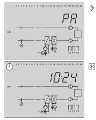
Switch to the configuration and parameter level. **PA** appears on the display.
