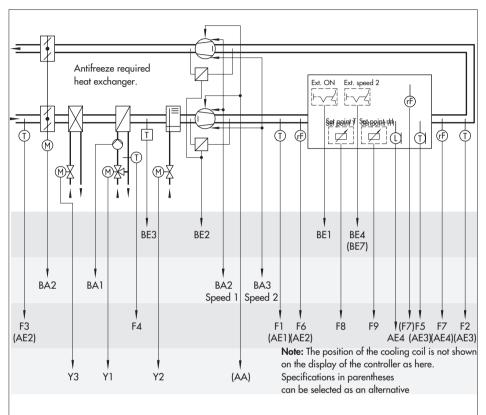
Fig. 10 · Anl 6 (system code no. 6) (air-conditioning, humidifying and dehumidifying)
