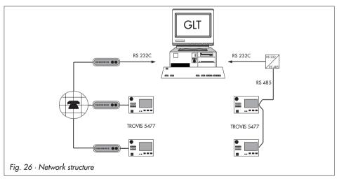
The TROVIS 5477 Ventilation Controller is equipped with either a RS-232-C or a RS-485 interface depending on the order. It is not possible to change the interface later.
