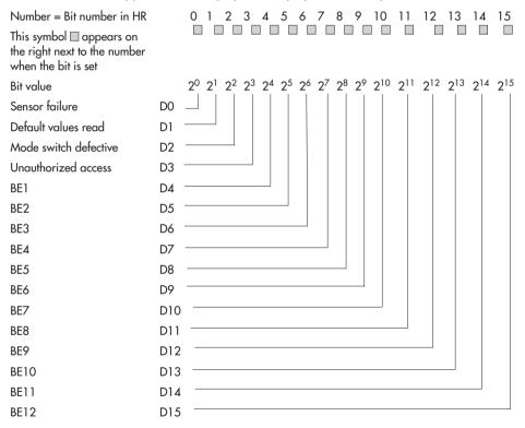
The binary inputs are registered in the status register when the function block associated with it is activated in the configuration level.
