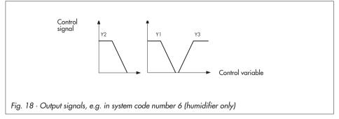
The operating action of the control output Y2 can be reversed.
