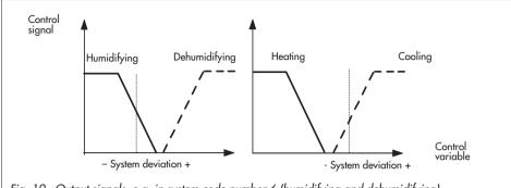
Fig. 19 · Output signals, e.g. in system code number 6 (humidifying and dehumidifying)
