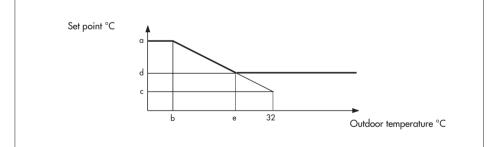
Fig. 22 · Outdoor temperature-compensated supply air control
