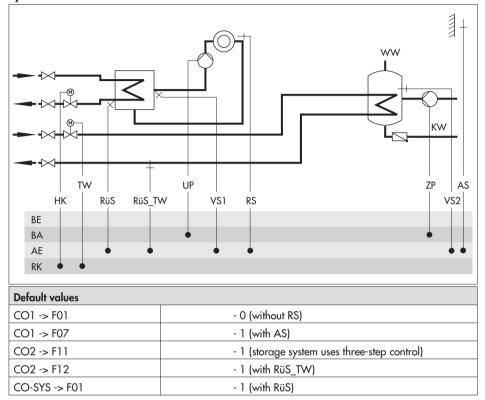
Using setting CO2 -> F11 - 0, a temperature valve is configured instead of the three-step control valve DHW.
