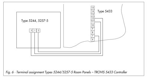
Apart from measuring the room temperature, the Type 5244 Room Panel (PTC sensor) and the Type 5257-5 Room Panel (Pt 1000 sensor) allow you to influence the control process as follows:
