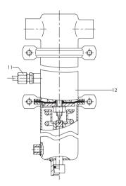
**Type M 44-7** · Set point ranges 0.02 to 0.12 bar · 0.1 to 0.5 bar · 0.3 to 1.1 bar 0.8 to 2.5 bar · 2 to 5 bar · 4 to 8 bar 6 to 12 bar
