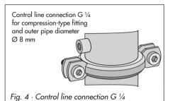
Use compression-type fitting with cylindrical male stud according to DIN 2353 for stainless steel pipes.
