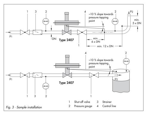
When tapping the pressure at a straight pipeline section, observe a minimum distance of at least six times the nominal valve size to the regulator.
